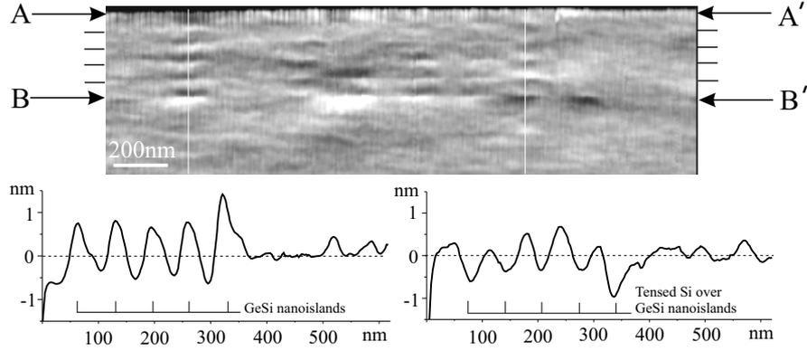
Figure 3: AFM topography image of the cleavage of 5-layered GeSi/Si heterostructure. A-A' line corresponds to edge of the sample. B-B' line corresponds to the first GeSi layer. Profiles demonstrate the details of a vertical alignment of 5 elevations (left) and 5 depressions (right). It is also seen an obvious up and down lifting of the Si matrix surface in between GeSi nanoislands.
