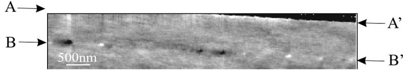
Figure 1: AFM topography image of GeSi/Si(001) structure cleavage. A-A' line corresponds to edge of the sample. B-B' corresponds to layer of GeSi nanoislands.
