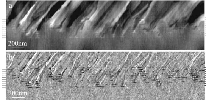
Figure 4: Topography image (a) and nanostiffness map (b) of GaSb layer with 10 layers of InSb quantum dots.
