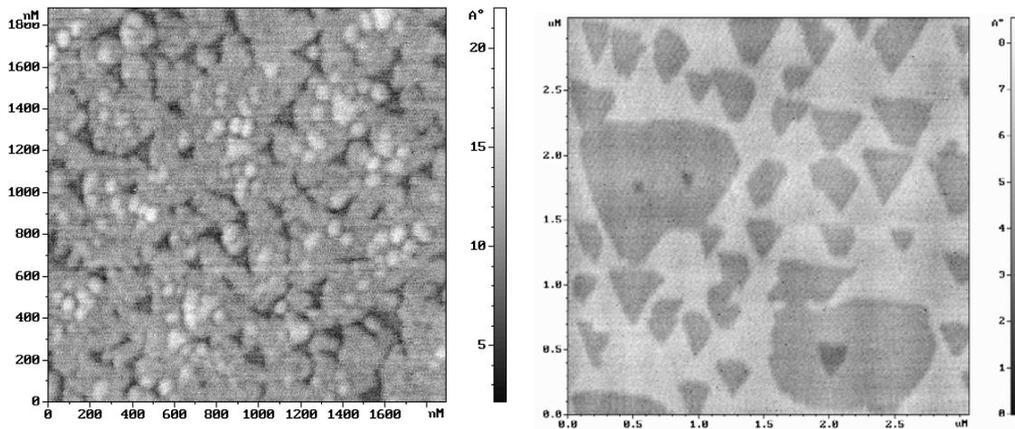
Fig.3. AFM-image of the silicon (111) surface after deposition of silicon atoms (a) and oxygen etching (b) at the condition of multilayer growth.
