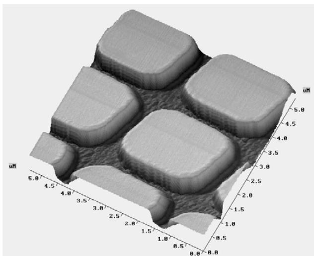
Fig.1. Three dimensional AFM-image of silicon (001) surface “meza”-structured by using optical lithography and chemical etching.
