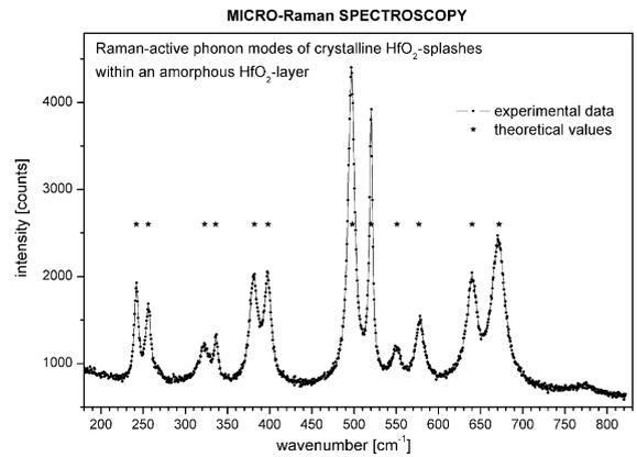
Fig. 5. Raman spectrum of a splash within a hafnium oxide layer. The very narrow and well-defined peaks indicate a good crystalline quality. Experimental results are in excellent agreement with theoretical values [15].
