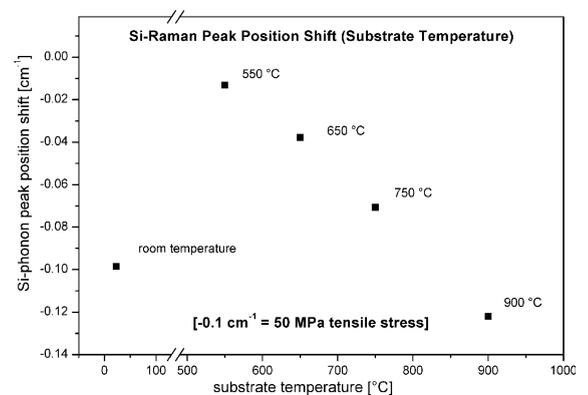
Fig. 6. Silicon Raman peak shift in dependence of growth temperature. All measurements indicate tensile stress while the magnitude of this stress changes with growth temperature.
