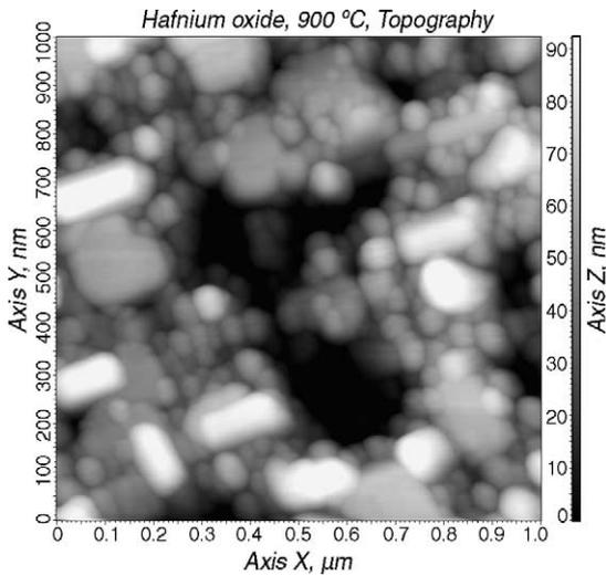
Fig. 4. Enlarged view of  $\text{HfO}_2$  layer grown at 900 °C substrate temperature.
