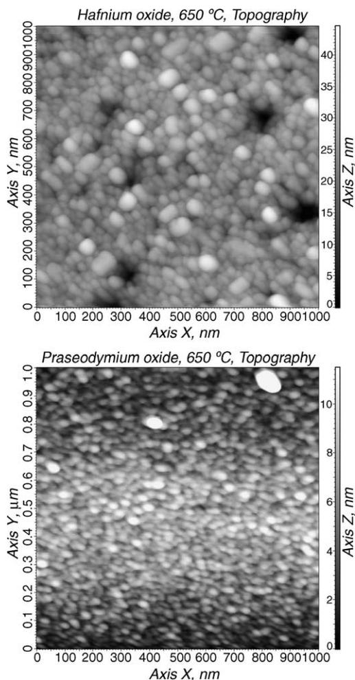
Fig. 2. AFM topography images of 10 nm thick  $\text{HfO}_2$  (top) and  $\text{Pr}_x\text{O}_y$  (bottom) films grown at 650 °C on Si(100). There are three features visible: small islands with a lateral size of around 40 nm in the background, bigger island with a size of 50 nm in the foreground and deep holes reaching the substrate. Note the change in amplitude by a factor of 4.
