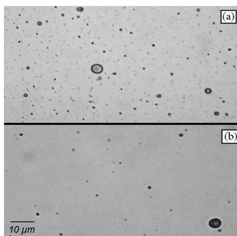
Fig. 1. Optical micrographs of 10 nm  $\text{Pr}_x\text{O}_y$  (a) and  $\text{HfO}_2$  (b) films on Si(100) showing the typical morphology. Both films were produced using a laser wavelength of 355 nm.
