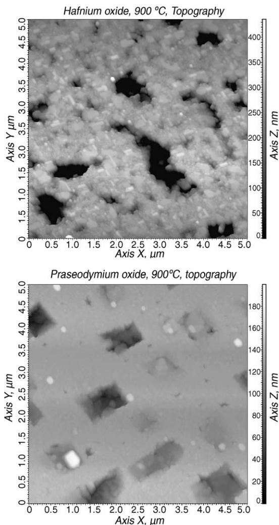
Fig. 3. AFM topography images of 10 nm thick  $\text{HfO}_2$  (top) and  $\text{Pr}_x\text{O}_y$  (bottom) films grown at 900 °C on Si(100). On  $\text{HfO}_2$  angular areas appear, indicating the formation of crystallites.
