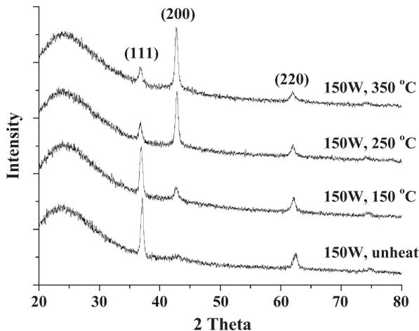
Fig. 3. XRD spectrum from the as-deposited NiO films prepared at RF power 150 W and different substrate temperatures.
