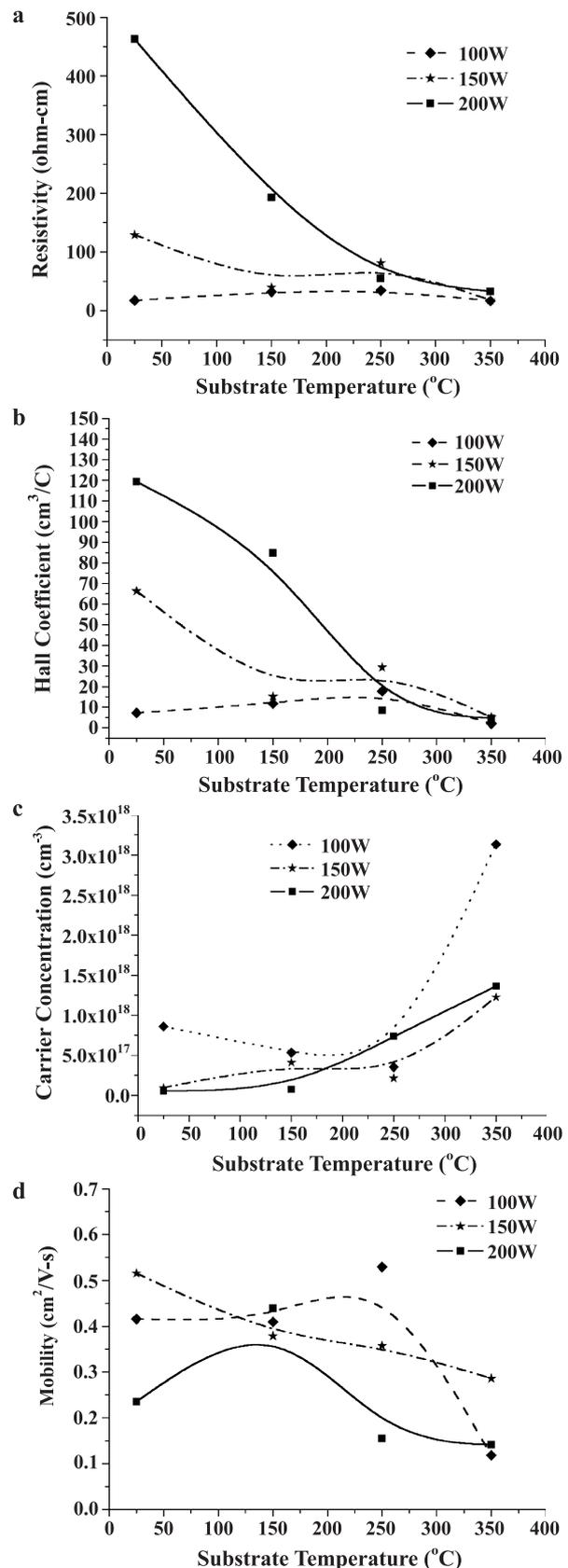
Fig. 5. Hall measurement of the nickel oxide films: (a) resistivity; (b) Hall coefficient; (c) carrier concentration; (d) mobility.
