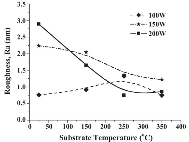
Fig. 2. Surface roughness of NiO films at different sputtering powers and substrate temperatures.
