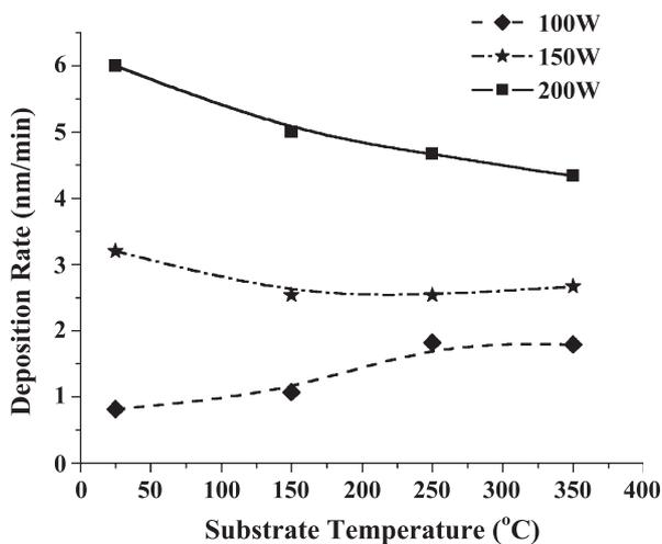
Fig. 1. Deposition rate of NiO films at different sputtering powers and substrate temperatures.
