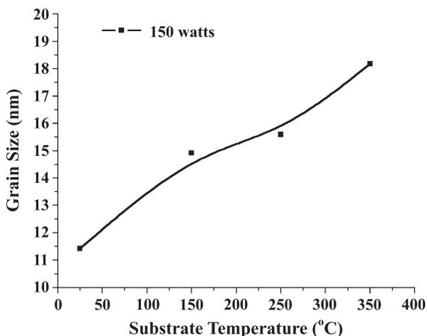
Fig. 4. The grain size of NiO films under various substrate temperatures at RF power 150 W.
