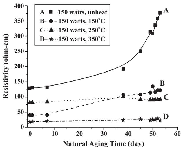
Fig. 6. The variation of resistivity of NiO films in natural aging test.
