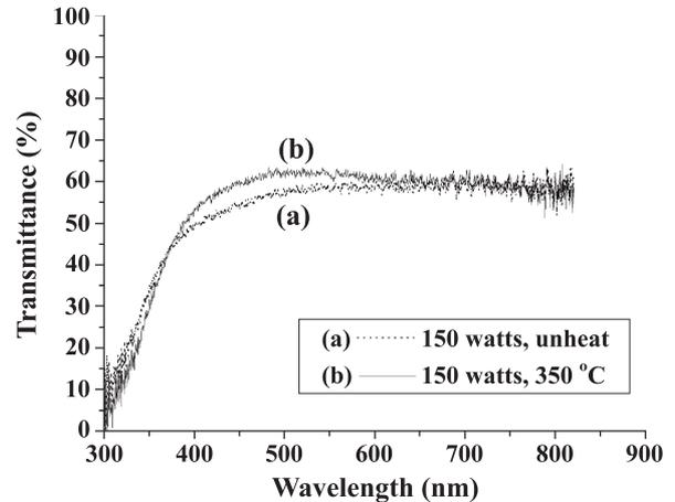
Fig. 7. The variation of spectral transmittance of the nickel oxide films at RF power 150 W and different substrate temperatures.
