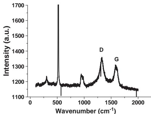
Fig. 4. Raman spectrum of nanotubes shown in Fig. 2(b) which were grown on a single NiO<sub>x</sub> square template of size 1.8 μm at 700 °C for 10 min.
