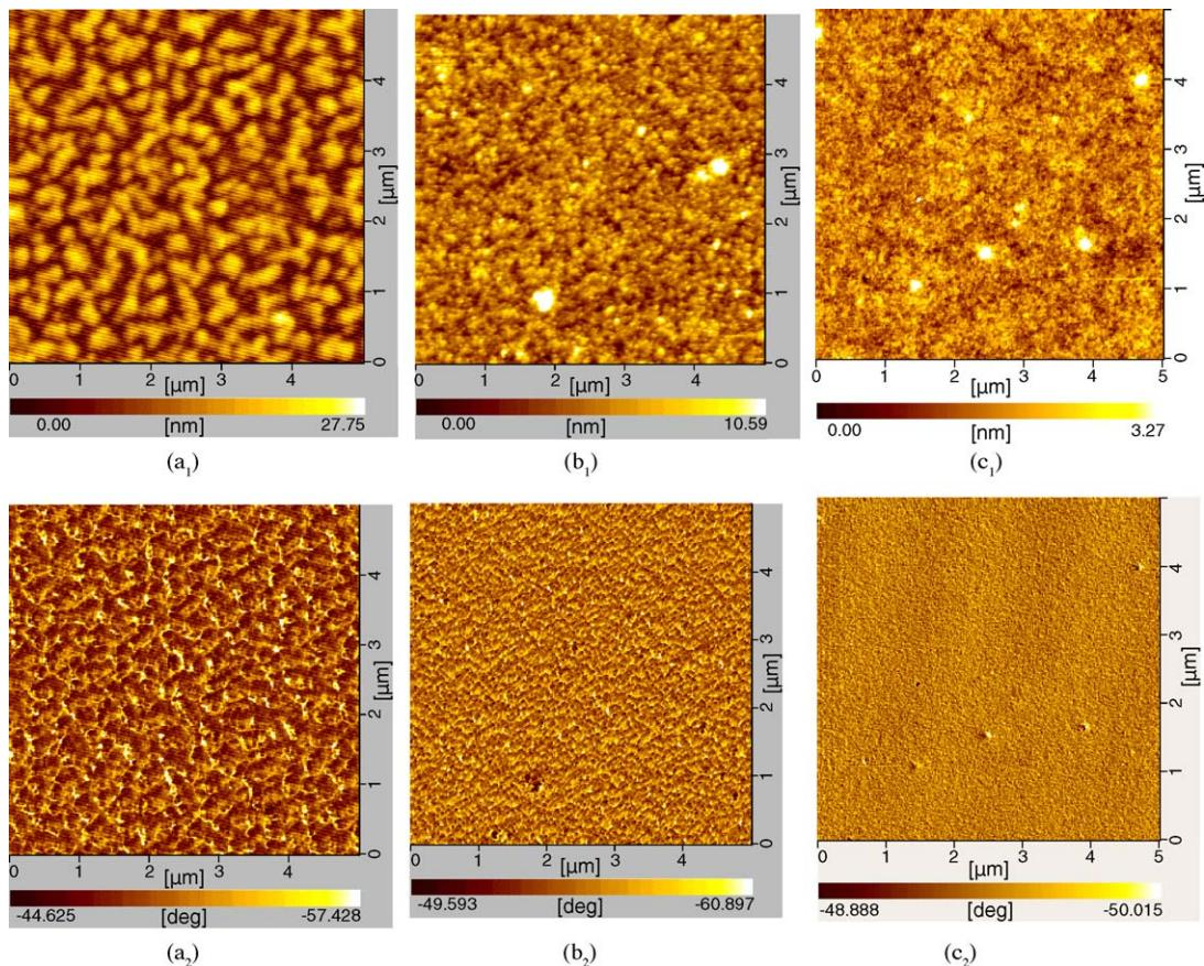
Fig. 1. The topographic and phase images of membranes. (a<sub>1</sub>–c<sub>1</sub>) The topographic images of SPEEKK, SPEEKK/PAN (0.5%), SPEEKK/PAN (1%). (a<sub>2</sub>–c<sub>2</sub>) The phase images of SPEEKK, SPEEKK/PAN (0.5%), SPEEKK/PAN (1%).
