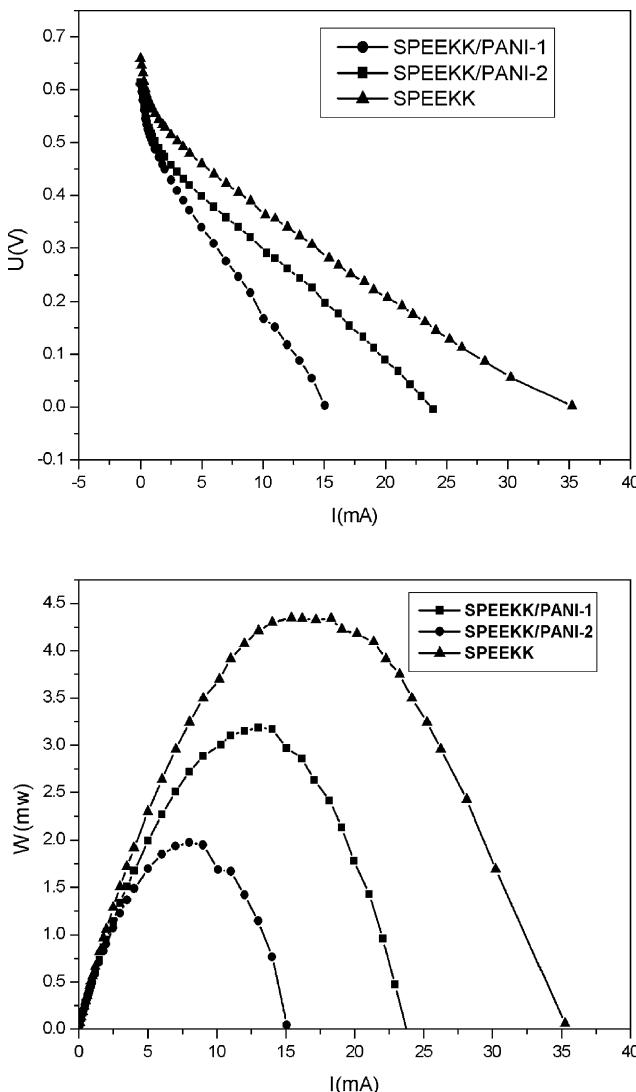
Fig. 6. The cell performance of SPEEK and its composite membranes.
