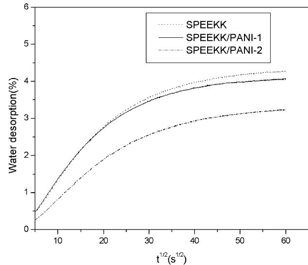
Fig. 5. Water desorption isotherm of membranes.
