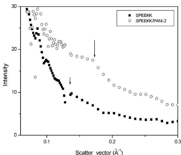
Fig. 2. The SAXS of SPEEKK and its composite membranes.
