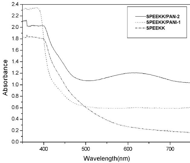
Fig. 4. UV curves of SPEEK and its composite membranes.
