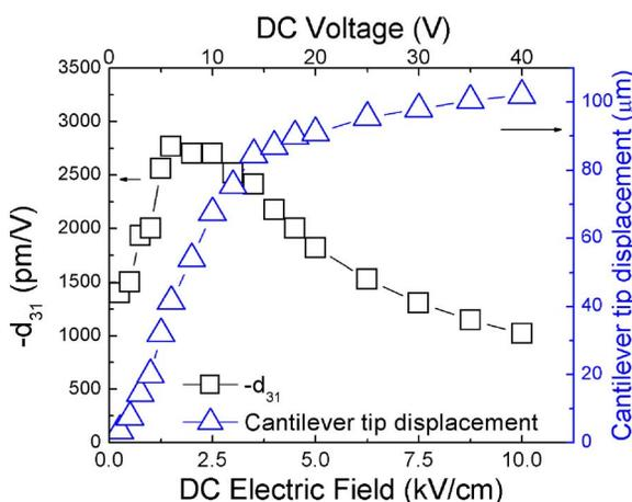
FIG. 4. (Color online)  $-d_{31}$  vs dc electric field of 40  $\mu\text{m}$  thick PMN-37PT freestanding films as deduced from the cantilever tip displacement measurement of a 4 mm long PMN-37PT/copper cantilever. Also shown is the tip displacement of the PMN-37PT/copper cantilever.
