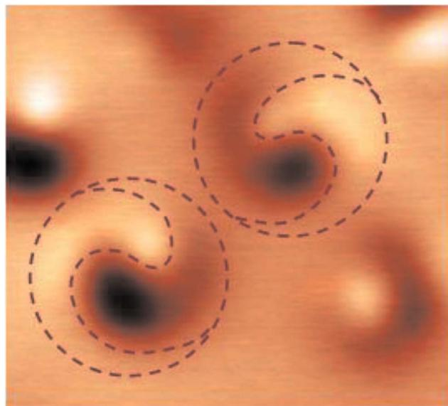
FIG. 6. (Color online) MFM image of two helical nanomagnets with different chirality. The frame size is  $1.8 \times 1.8 \mu\text{m}$ .
