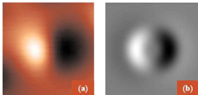
FIG. 4. (Color online) (a) Experimental and (b) simulated MFM contrast distributions for a triple nanodisk with equal Co thicknesses.
