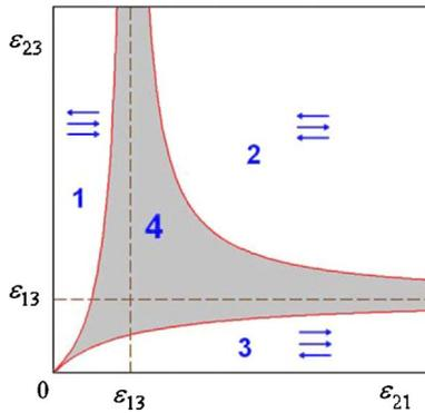
FIG. 2. (Color online) The diagram of states in triple nanodisk. The central region 4 (indicated in gray color) corresponds to the noncollinear states.
