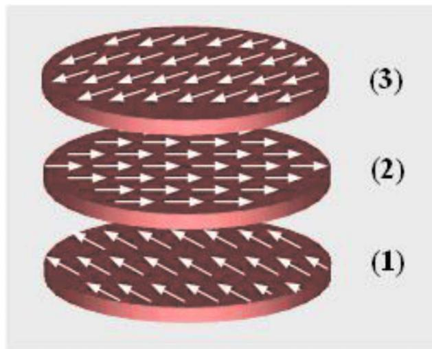
FIG. 1. (Color online) Noncollinear helical magnetic state in the three single-domain disks system.
