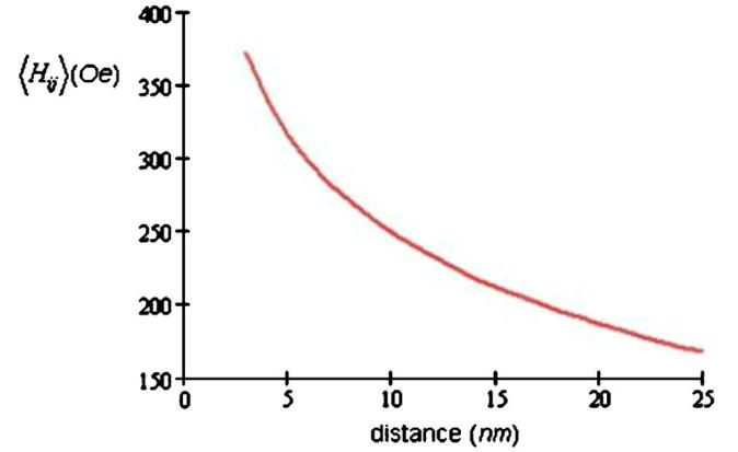
FIG. 3. (Color online) Dependence of volume averaged longitudinal component of the magnetic field with the distance between the disks  $z_{ij}$ .
