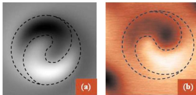
FIG. 5. (Color online) (a) Model MFM contrast distribution for optimized triple nanodisk. (b) Experimental MFM image from triple 16, 11, and 8 nm Co nanodisk. (Frame size  $1 \times 1 \mu\text{m}$ .) The dashed lines separate the regions with dark and bright contrast to emphasize the spiral symmetry of MFM contrast.
