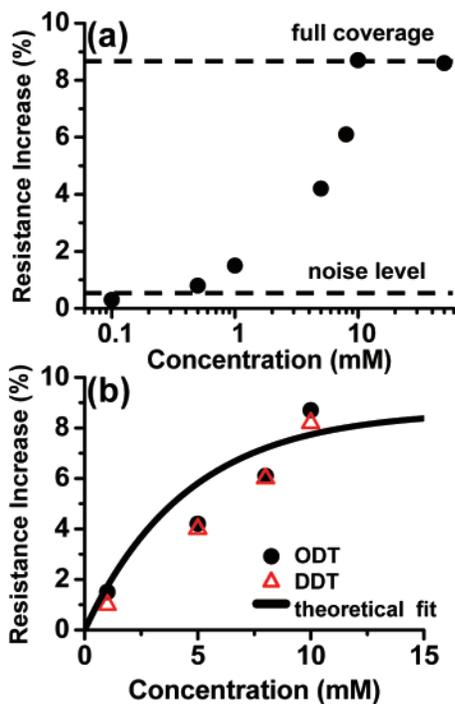
**Figure 7.** (a) The relationship between the resistance increase and the ODT concentration for an immersion time of 5 min. (b) The relationships between the resistance increase and the concentration in the range between 1 and 10 mM for ODTs and DDTs and a theoretical fit based on eq 4.
