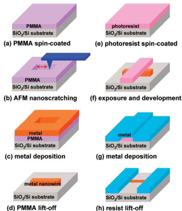
**Figure 1.** A schematic diagram of the fabrication of a metal nanowire connected with metal electrodes.
