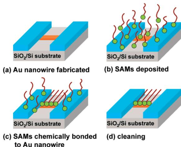
**Figure 2.** A schematic diagram of the procedure for establishing chemical binding between the SAMs and an Au nanowire.
