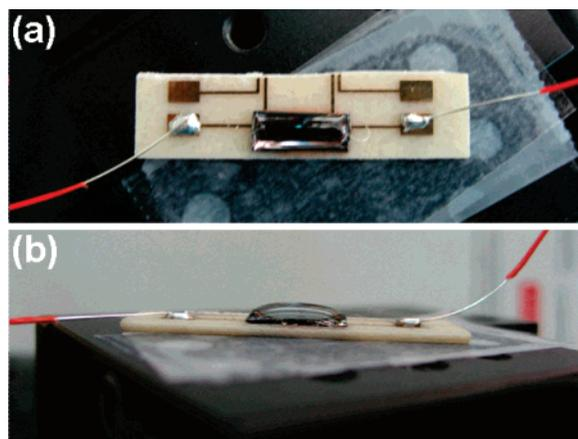
**Figure 3.** (a) Top-view and (b) side-view photographs of a resistance measurement unit. Note that in part b an excess amount of SAM solution is deposited for visual effect.
