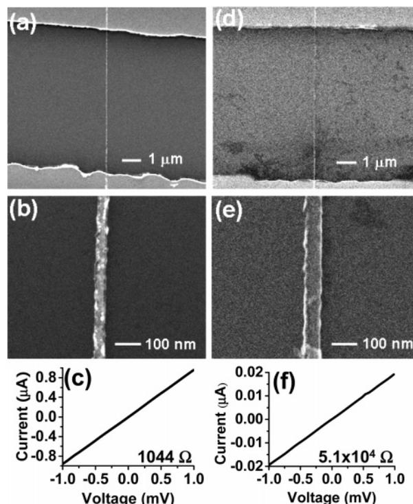
**Figure 4.** SEM images of (a) Au and (d) Ti nanowires connected with Au and Ti electrodes, respectively. Zoomed images of (b) the Au and (e) the Ti nanowires. (c) and (f) The corresponding  $I$ – $V$  curves of the nanowires in parts a and d, respectively.
