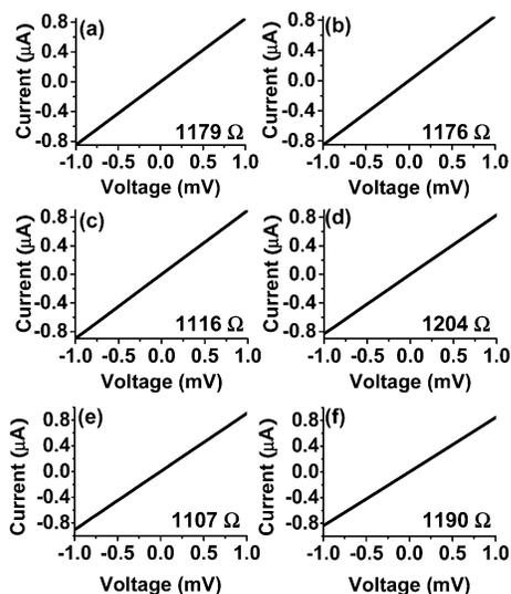
**Figure 6.** The  $I$ - $V$  curves of Au nanowires (a) before and (b) after the deposition of absolute alcohol, (c) before and (d) after the deposition of a 10 mM ODT solution, and (e) before and (f) after the deposition of a 10 mM DDT solution.
