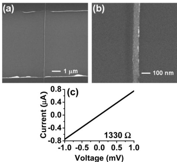
**Figure 5.** (a) SEM image of an Au nanowire connected with Ti electrodes, (b) a zoomed image of the Au nanowire, and (c) the corresponding  $I$ - $V$  curve.
