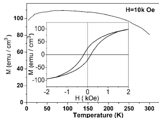
FIG. 4. Temperature-dependent magnetization curve of chromium oxide nanoparticle film measured at 10 kOe. (Inset) magnetic hysteresis loop taken at 5 K.
