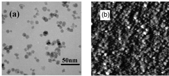
FIG. 1. (a) TEM image of a typical low coverage deposit sampled on an amorphous carbon film of TEM grid with short deposition time. (b)  $1600 \times 1600 \text{ nm}^2$  AFM image of a heavily deposited film sampled on a flat silica glass sheet.
