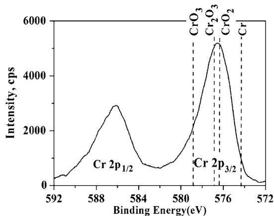
FIG. 2. XPS Cr  $2p$  core level spectrum of the chromium oxide nanoparticle assembled film. Vertical dash lines indicate binding energies of chromium oxides  $\text{CrO}_3$  (578.8 eV),<sup>11</sup>  $\text{CrO}_2$  (576.3 eV),<sup>12</sup>  $\text{Cr}_2\text{O}_3$  (576.8 eV),<sup>12</sup> and metallic chromium (574.3 eV).<sup>11</sup>
