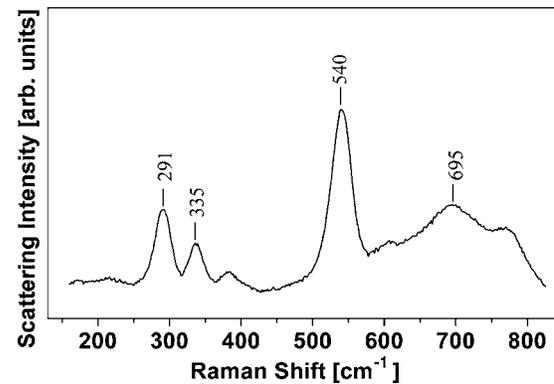
FIG. 3. Raman spectrum of the chromium oxide nanoparticle assembled film.
